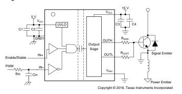
Figure 3. Inverting Configuration
