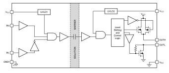
Figure 2. Gate Driver Function Block Diagram
