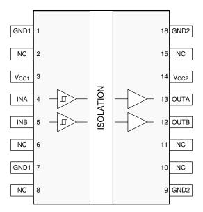
Figure 4-2. Pin Diagram (16-DW Package)
