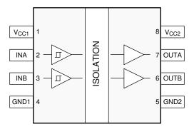
Figure 4-1. Pin Diagram (8-D) Package
