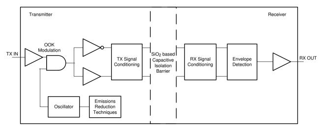
Figure 1-1. Functional Block Diagram
