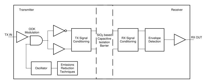
Figure 1-1. Functional Block Diagram
