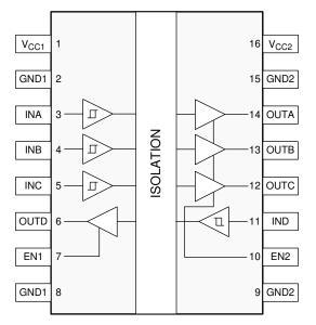
Figure 4-1. Pin Diagram (common for all 3 Packages)
