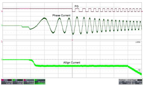
Figure 2-2. Phase Current and FG During Align
