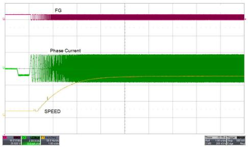
Figure 2-12. FG, Phase Current and Motor Electrical Speed in Hz With Manually Tuned Kp and Ki
