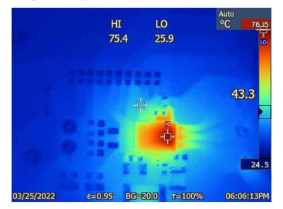
Figure 2-15. Thermal Image of MCF8316A - Lower Case Temperature
