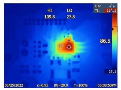
Figure 2-14. Thermal Image of MCF8316A – Higher Case Temperature
