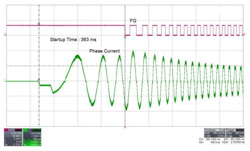
Figure 2-3. Time Taken to Enter Closed Loop in Align
