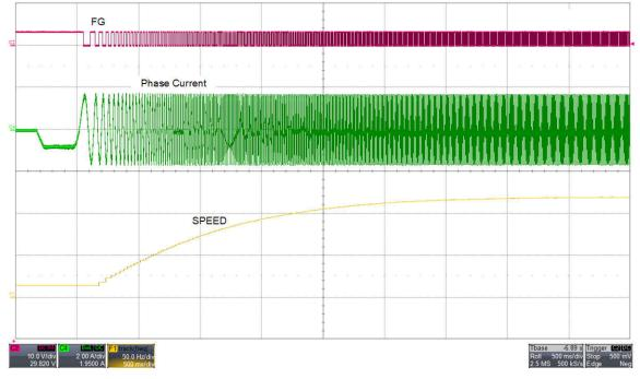
Figure 2-11. FG, Phase Current and Motor Electrical Speed in Hz With Auto Tuned Kp and Ki
