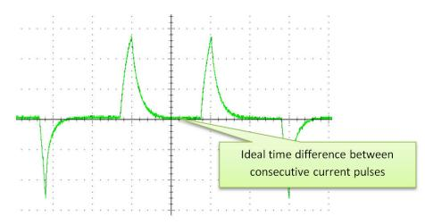
Figure 2-6. IPD Current Pulses Showing Ideal IPD Clock Frequency
