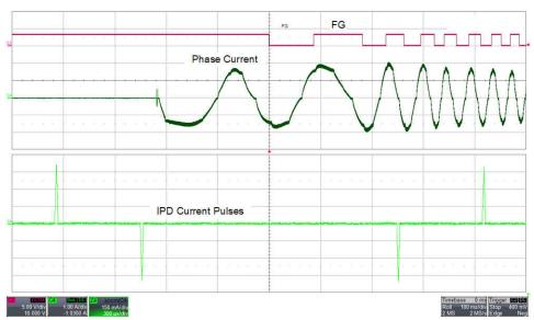
Figure 2-7. Phase Current and FG During IPD
