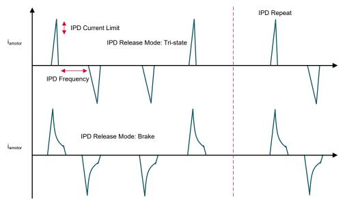
Figure 2-4. IPD Current Pulses in Tri-State and Brake Mode
