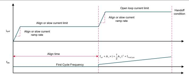
Figure 2-1. Q-Axis Current and Motor Electrical Frequency During Align
