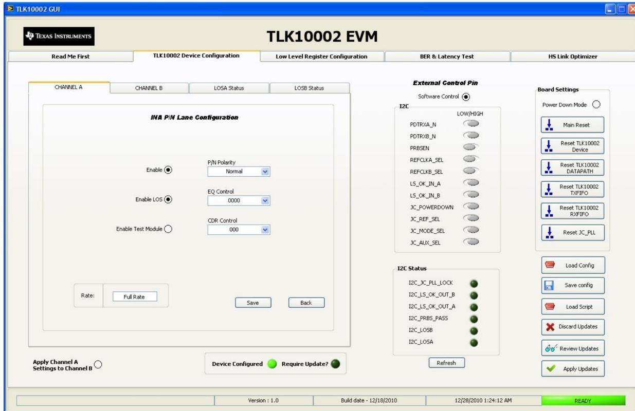
**Figure 5. TLK10002EVM GUI High-Level Device INAP/N Configuration**
