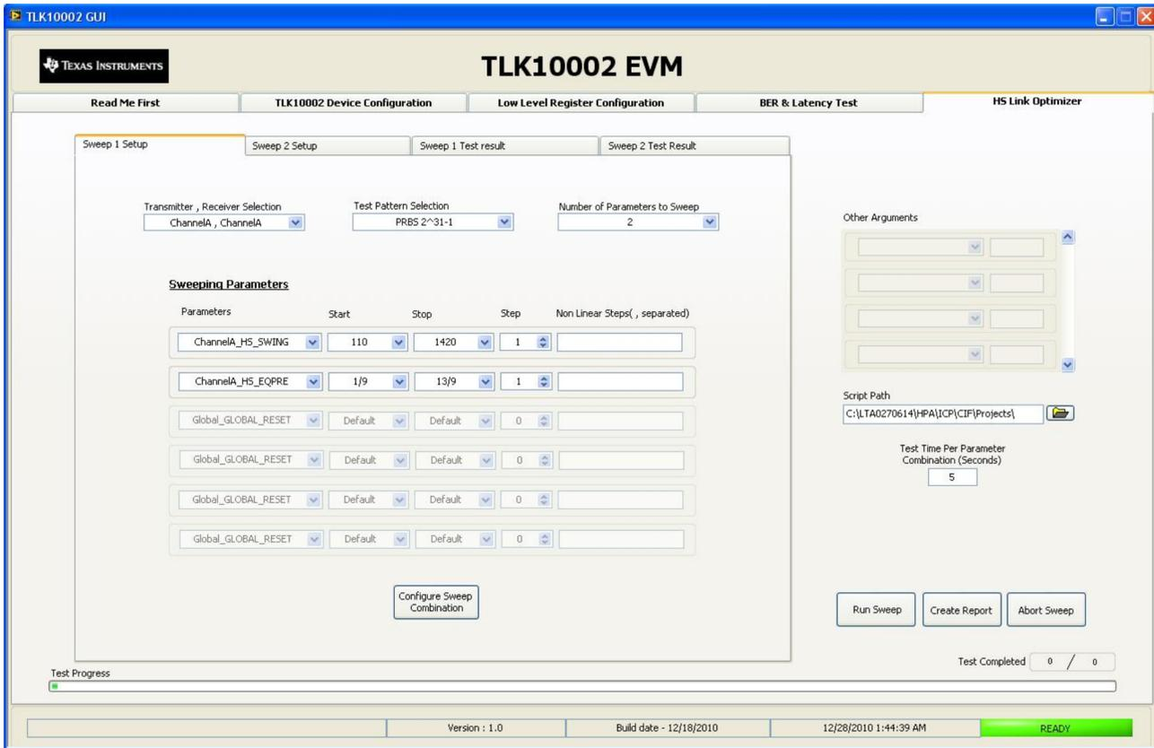
**Figure 19. TLK10002EVM GUI High-Speed Link Optimizer Tab**
