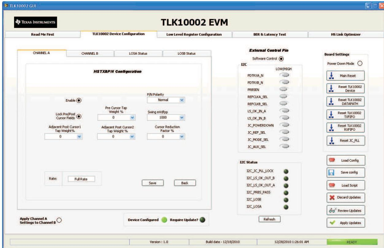
**Figure 7. TLK1002EVM GUI High-Level Device HSTXAP/N Configuration**
