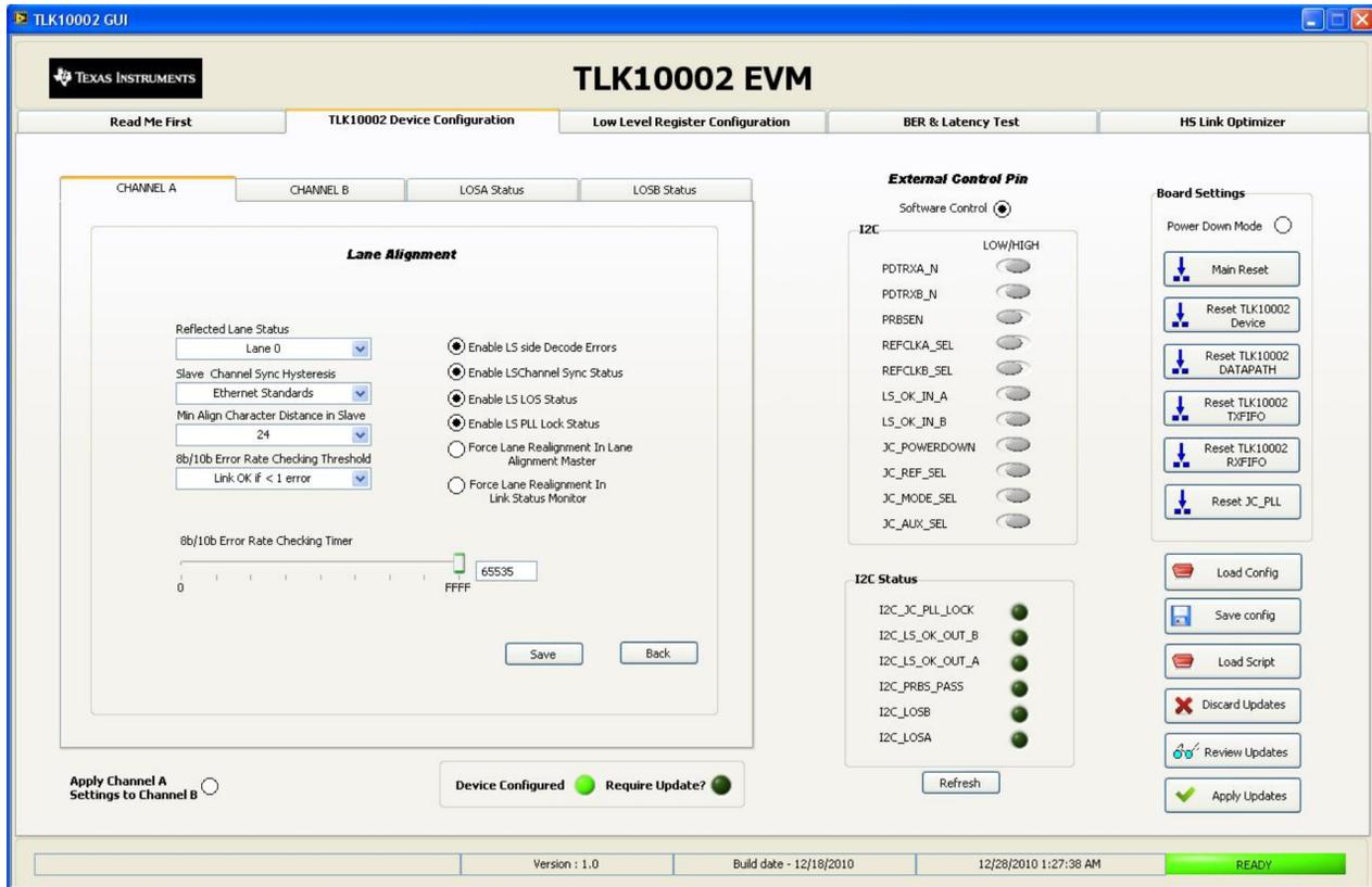
Figure 10. TLK10002EVM GUI High-Level Device Lane Alignment Configuration
