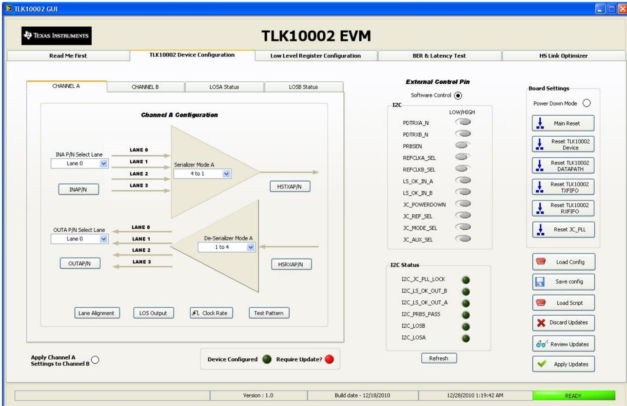
Figure 3. TLK10002EVM GUI High-Level Device Configuration Window
