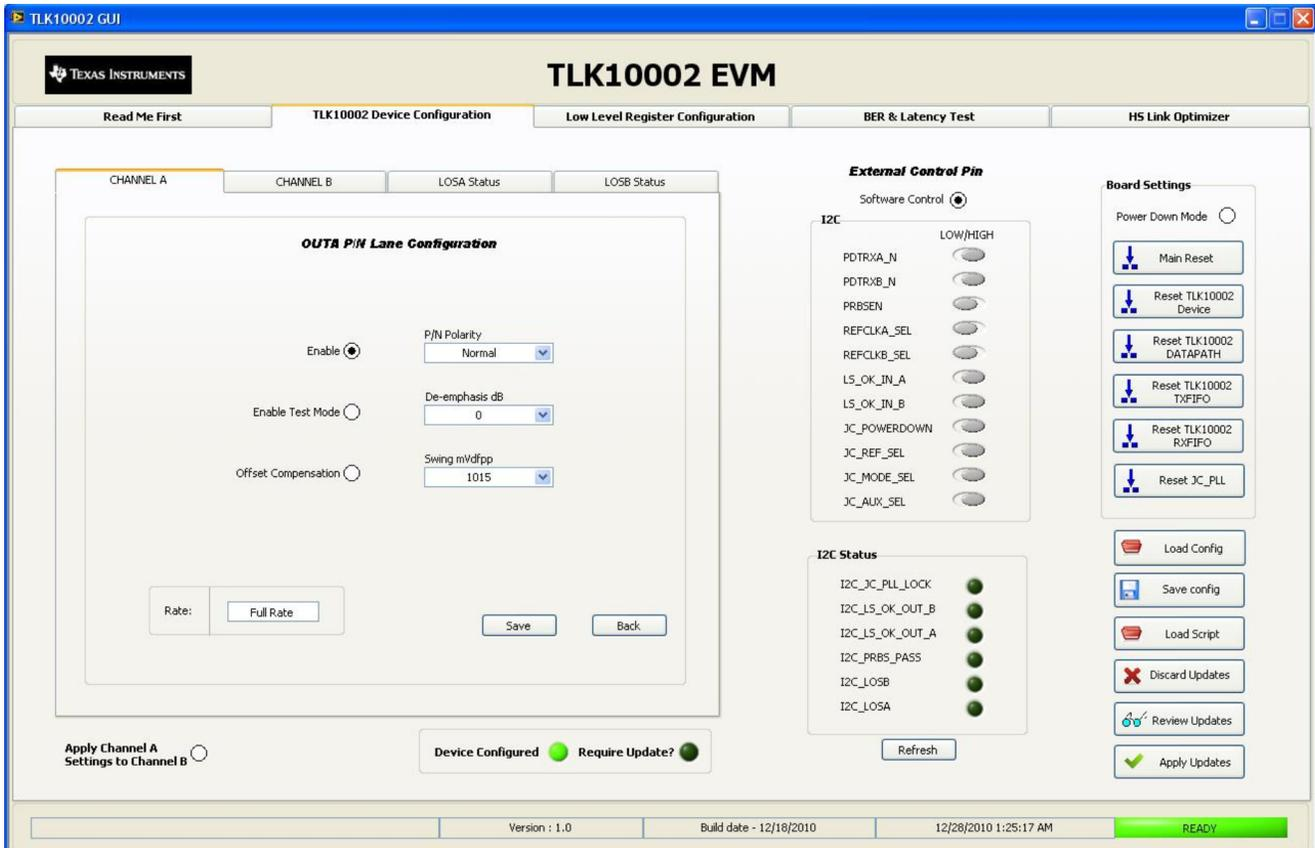
Figure 6. TLK10002EVM GUI High-Level Device OUTAP/N Configuration
