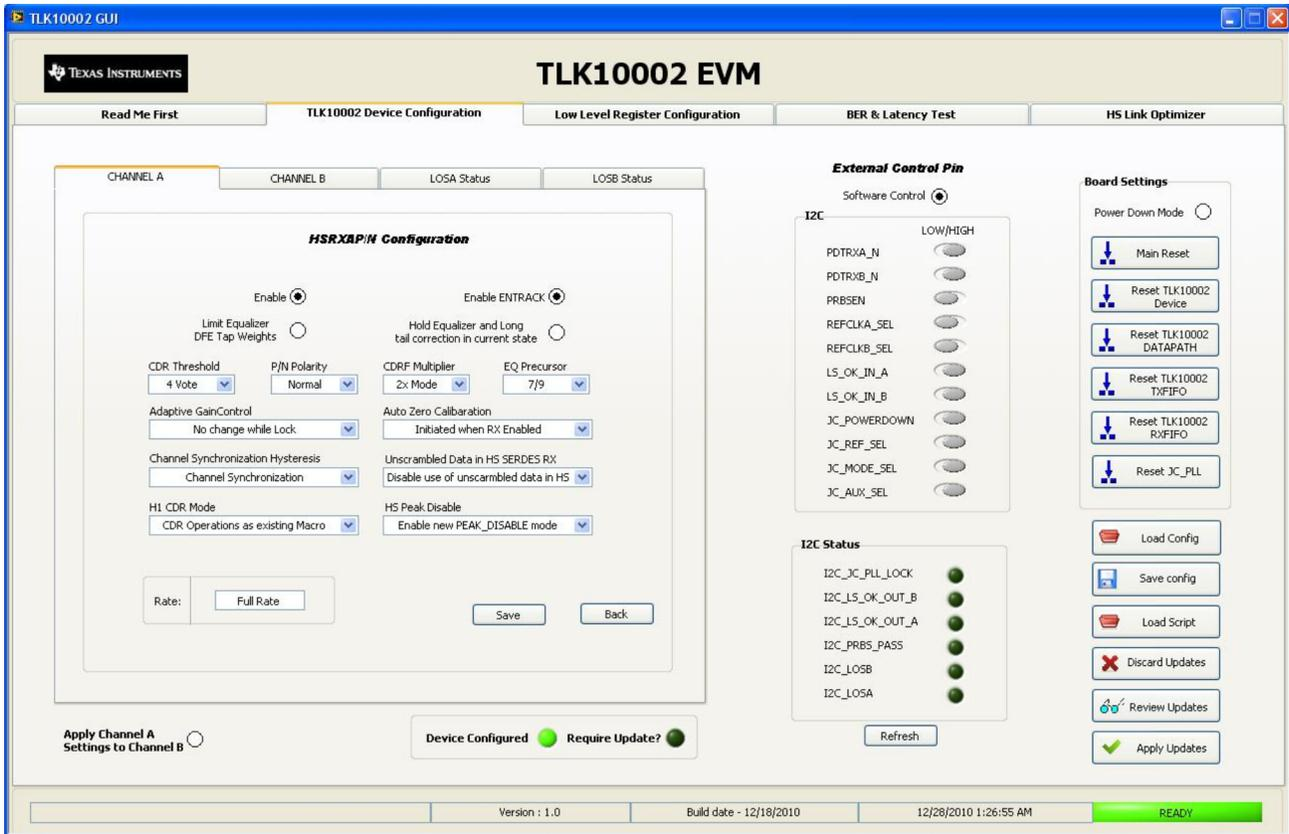
Figure 8. TLK10002EVM GUI High-Level Device HSRXAP/N Configuration
