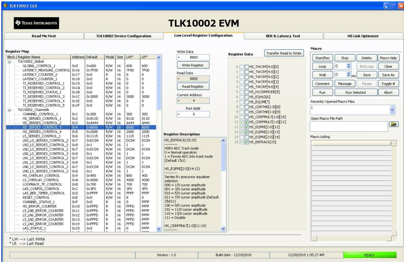
Figure 15. TLK10002EVM GUI Low-Level Register Configuration Window
