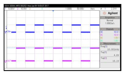
Figure 6. UCC53x0M Device Input and Output
