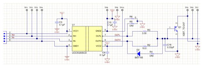
Figure 4. UCC53x0S EVM Signal Path Schematic
