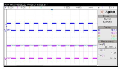
Figure 5. UCC53x0S Device Input and Output
