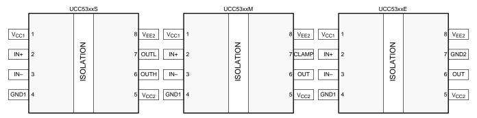
Figure 1. UCC53x0x Pin Configurations
