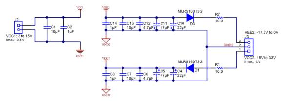
Figure 2. UCC53x0 EVM Power Supply Schematic
