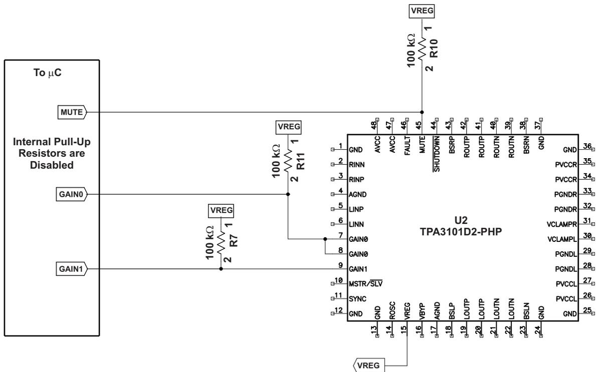
Figure 3. Alternate Method Number 1 – Circuit Diagram
