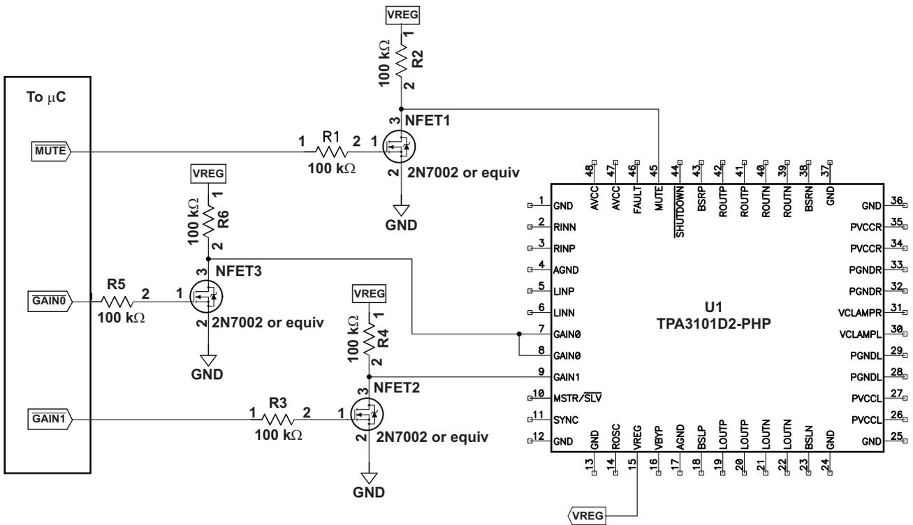
Figure 2. Connection to Amplifier (All Three Circuits Shown)
