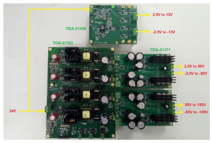
Figure 4. Combining TI Designs (Boards)
