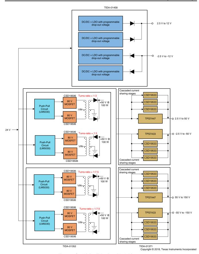
Figure 3. Combining TI Designs Block Diagram
