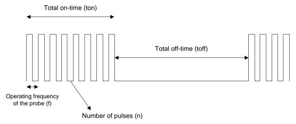
Figure 1. Standard Driving Waveform for Ultrasound Transducers
