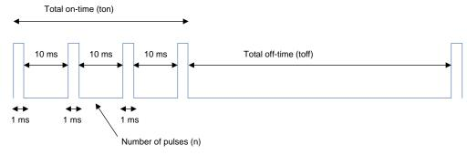
Figure 2. Elastography—Driving Waveform for Ultrasound Transducers
