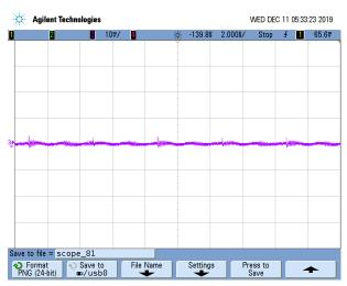
Figure 3-4. Output Ripple of Negative Rail After Power Filter
