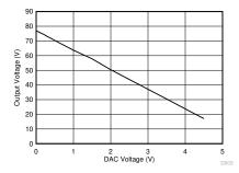
Figure 4-2. Linearity of Output Voltage vs Control Voltage (VDAC)
