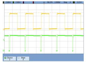
Figure 6-2. Synchronization at No Load With 50% Duty Cycle Clock
