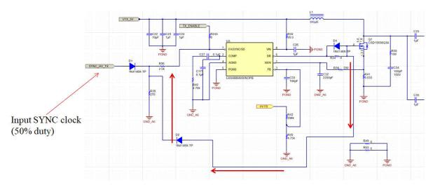
Figure 6-1. Section of the Schematic of HV Supply Updated After Implementation of SYNC Functionality
