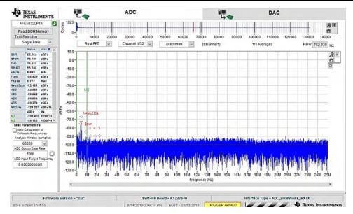
Figure 3-10. 11 FFT of the Received Data Using SEPIC Power Supply, Showing SNR of 55.264 dB
