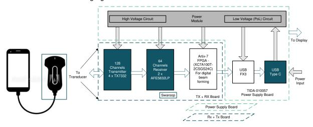
Figure 1-1. (left) Generic Smart Probe; (right) System Block Diagram of Smart Probe Ultrasound Scanner
