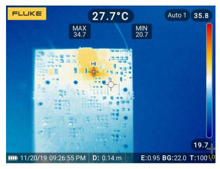
Figure 3-11. Thermal Performance of High Voltage Section
