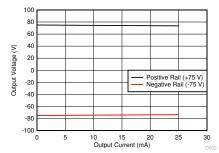
Figure 3-2. Load Symmetry of SEPIC Showing Accuracy of Less Than 1% and Load Regulation Less Than 2%
