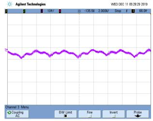
Figure 3-3. Output Ripple of Negative Rail Before Power Filter
