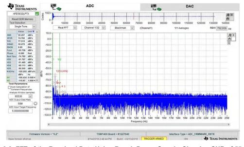
Figure 3-9. FFT of the Received Data Using Bench Power Supply, Showing SNR of 55.297 dB
