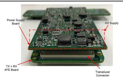
Figure 1-2. Power Supply and TX+RX AFE Boards
