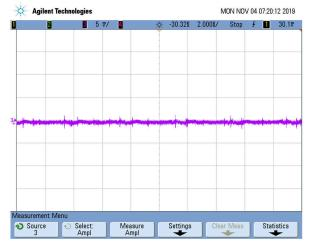
Figure 3-6. Output Ripple of Positive Rail After Power Filter
