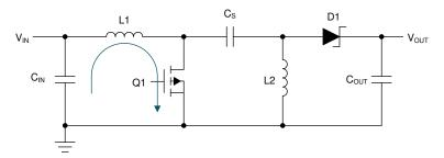
Figure 5-1. Hot Loop in SEPIC Configuration
