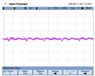
Figure 3-5. Output Ripple of Positive Rail Before Power Filter
