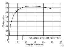
Figure 3-1. Efficiency Curve of SEPIC HV Power Supply
