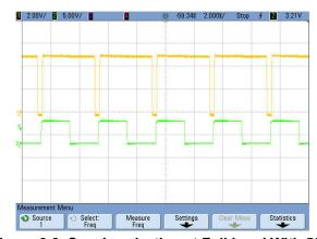
Figure 6-3. Synchronization at Full Load With 50% Duty Cycle Clock
