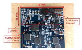
Figure 2-3. Power Supply Board Highlighting the HV Section
