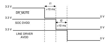
Figure 3. Line Driver Power Sequence
