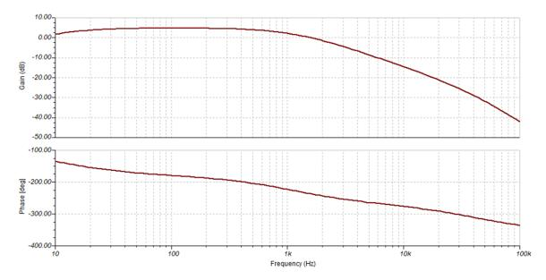
Figure 11. Frequency Response of Termination Resistor 270Ω. Increase the Feedback Resistor Values but Keep the Same Gain Level
