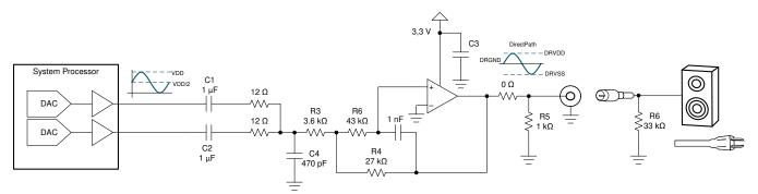
Figure 2. Subwoofer Line Driver Stereo to Mono Design
