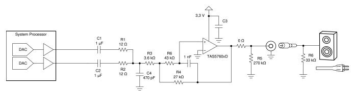
Figure 7. Subwoofer Line Driver Stereo to Mono Design With Output Impedance 270Ω Resistor
