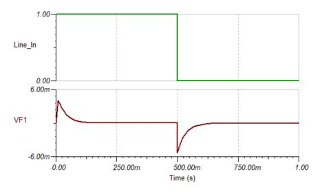
Figure 9. Step Response of Typical Subwoofer Line Driver Stereo to Mono Circuit
