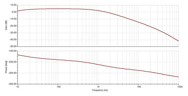
Figure 8. Frequency Response of Typical Subwoofer Line Driver Stereo to Mono Circuit
