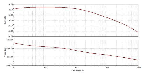
Figure 4. Frequency Response of Typical Subwoofer Line Driver Stereo to Mono Circuit
