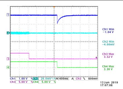
Figure 14. Increasing Line Driver Feedback Resistor Network's Waveform With 270  $\Omega$  Termination Resistor
