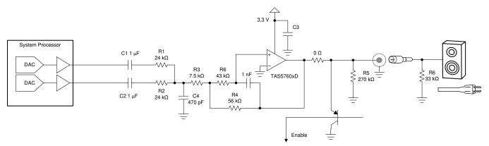
Figure 15. System Processor Control External BJT Before System Turns Off
