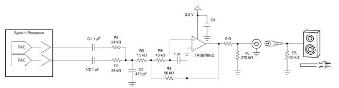
Figure 10. Subwoofer Line Driver Stereo to Mono Design With Output Impedance 270Ω Resistor and Twice Feedback Network Resistor
