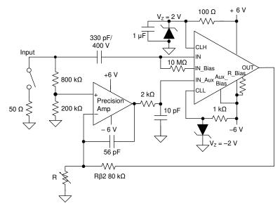
Figure 1. Example BUF802 Composite Loop Configuration
