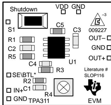
Figure 3–3. TPA311 EVM Schematic Diagram
