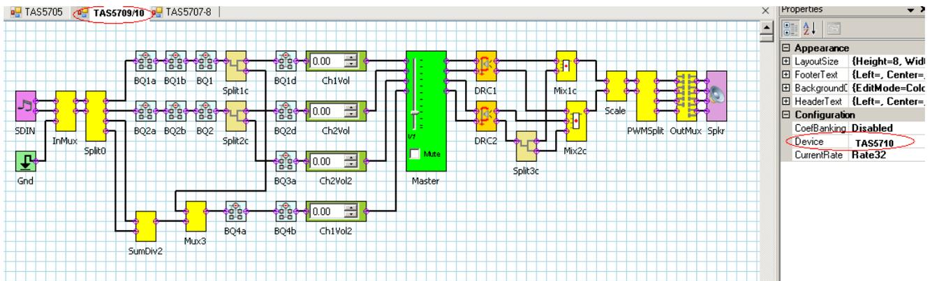
Figure 7. Process Flow for TAS5710 UG
