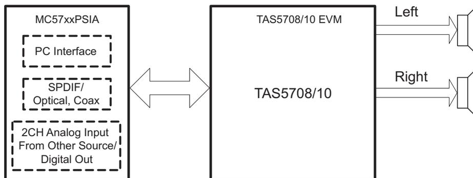
**Figure 2. Complete System and EVM Signal Path Overview**
