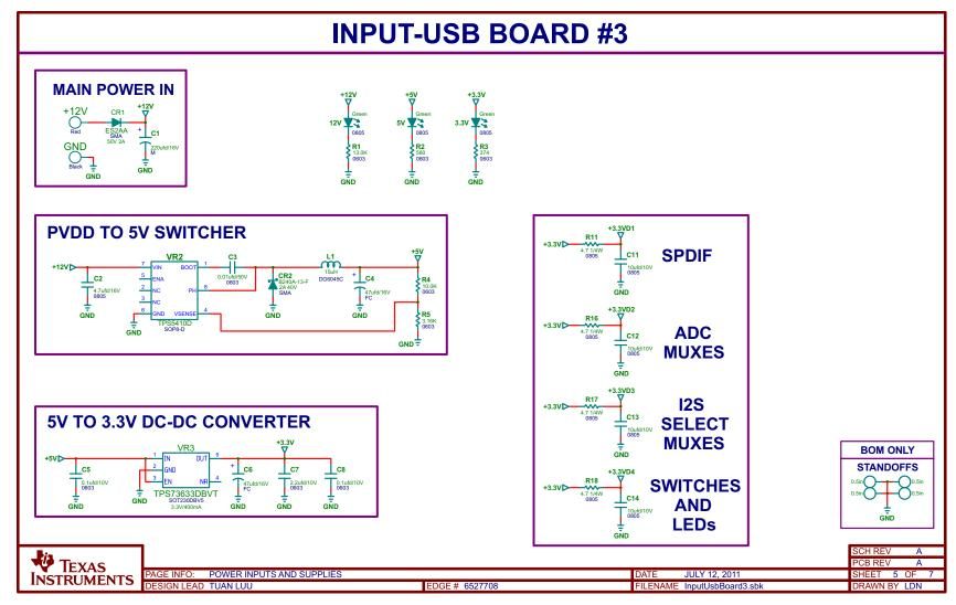
Figure 11. Input - USB Board3 Power Inputs and Supplies
