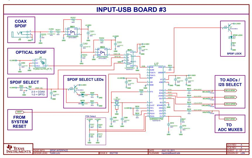
Figure 8. Input - USB Board3 SPDIF Interface
