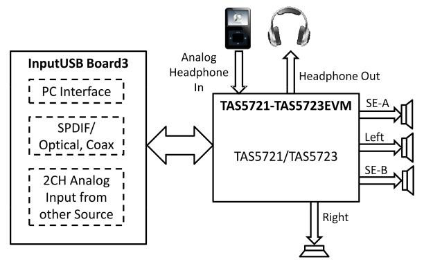
Figure 1. Complete System and EVM Signal Path Overview
