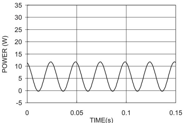
**Figure 6b. Instantaneous Output Power for Ring Generator (5 REN, Vos = 0V)**
