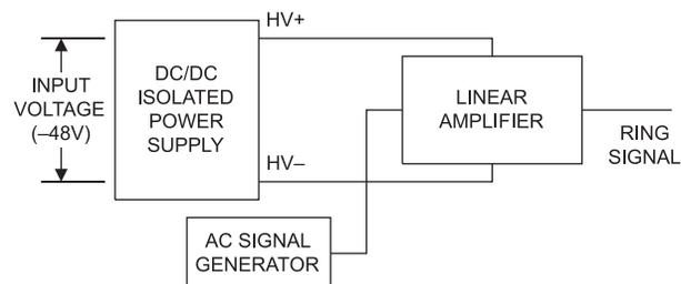
**Figure 1a. Conventional Ring Generation Using Linear Amplifier**
