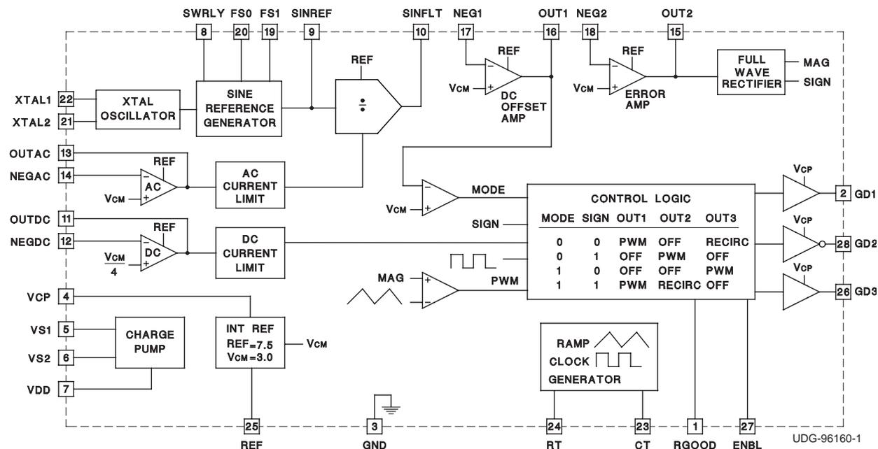
Figure 7. Block Diagram of the UCC3750
