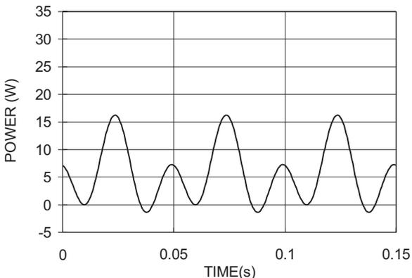
**Figure 6a. Instantaneous output power for ring generator (5 REN, Vos = -48V)**
