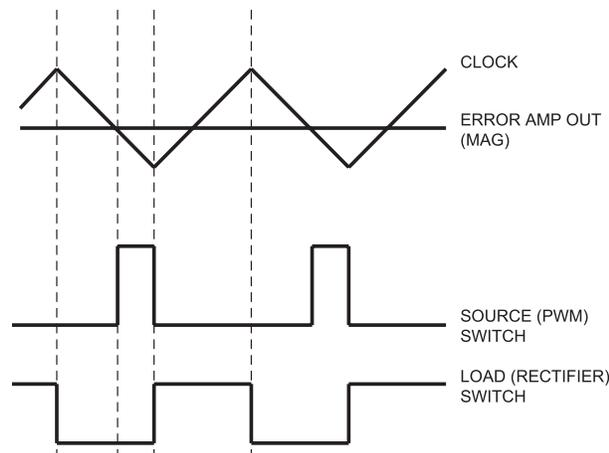
Figure 4. Circuit Waveforms (Switching Frequency)
