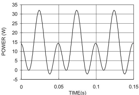
**Figure 6c. Instantaneous Output Power for Ring Generator (10 REN, Vos = -48V)**
