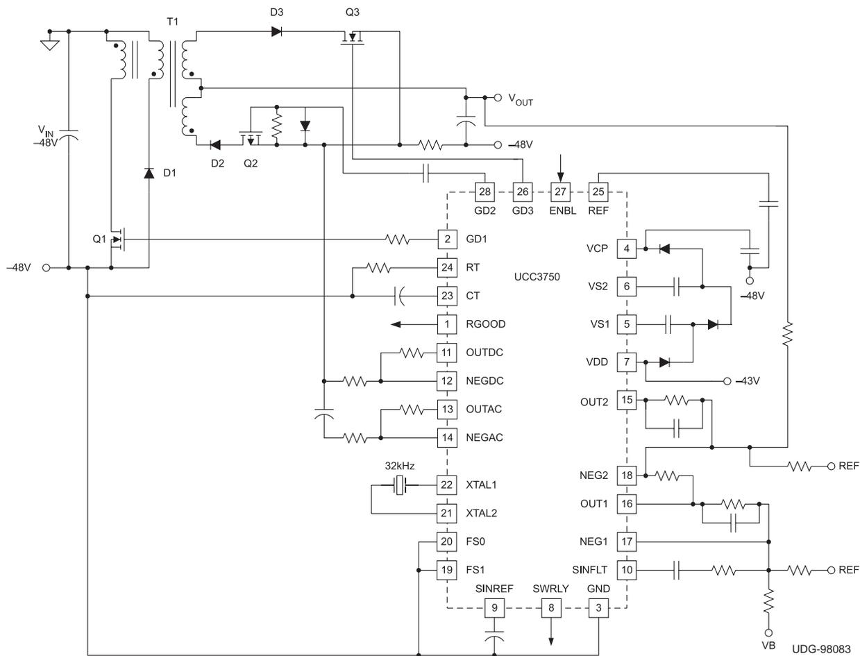
Figure 11. Non-isolated Ring Generator Implementation
