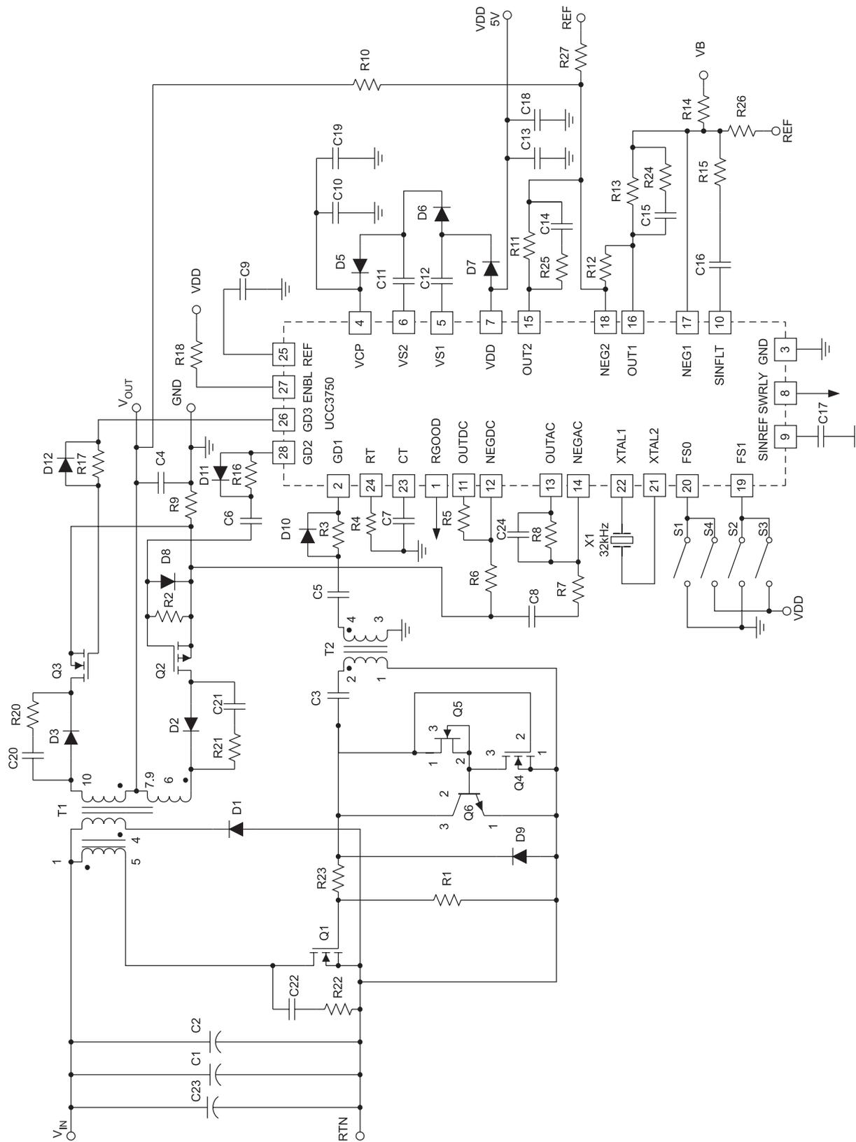
Figure 9. UCC3750 Detailed Application Circuit Schematic
