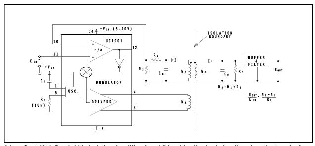
A Low Cost, High Bandwidth, Isolation Amplifier: An additional feedback winding linearizes the transfer function of the amplifier by matching the coupling characteristics to the isolated output.
