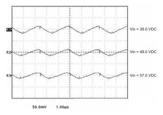
Figure 13. Output Ripple for Ethernet Input
