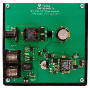
Figure 2. Building Power PD Demo Board
