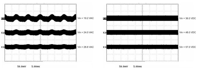
Figure 15 shows the output noise of the reference design at maximum load over the 36 VDC to 57 VDC range of the 48 VDC Ethernet input.
