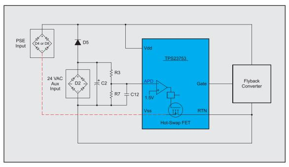
Figure 6. Simplified Block Diagram of Reference Design Priority Method
