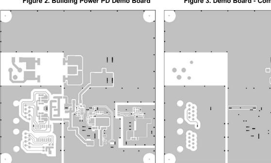
Figure 5. Demo Board – Bottom Copper
