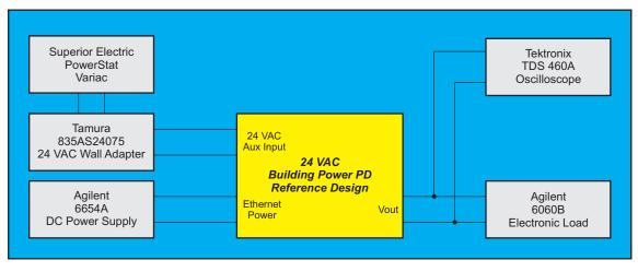
Figure 7. Simplified Block Diagram of Reference Design Test Setup
