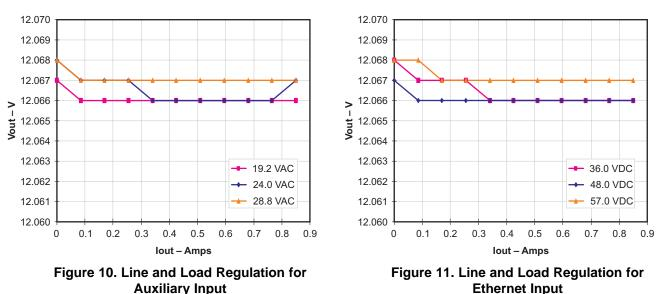
Figure 11 shows the line and load regulation of the reference design over the 36 VDC to 57 VDC range of the 48 VDC Ethernet input.
