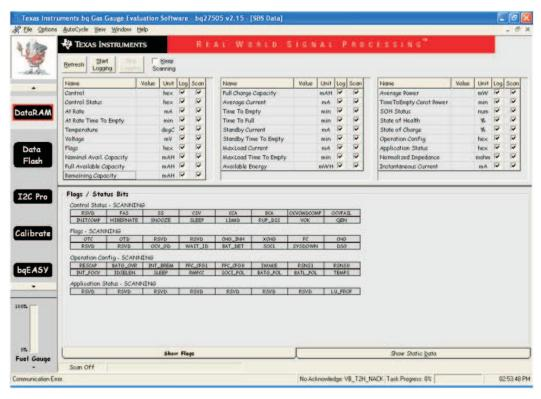
Figure 5. DataRAM Window Displaying No EV2300 Communication
