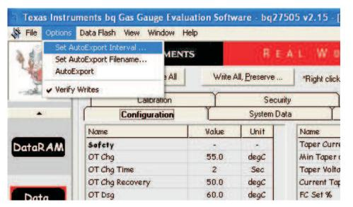
Figure 17. Gas Gauge Logging Setup and Start Commands
