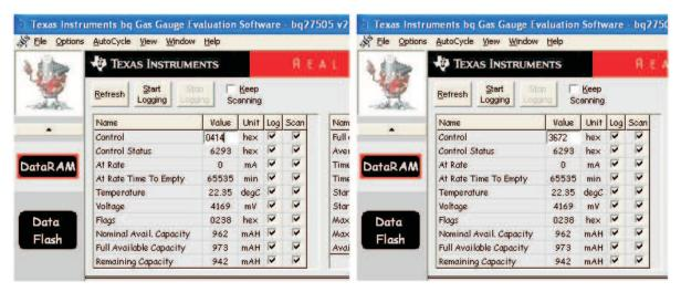
Figure 20. Default Unseal Command Using Control Register
