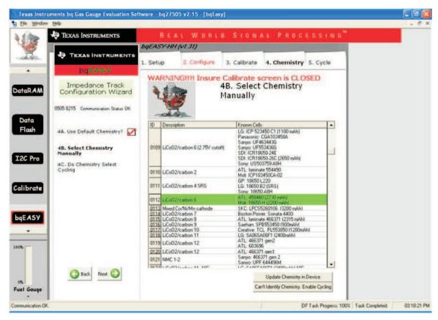
A unique chemical ID indicates a different battery chemistry being used.
