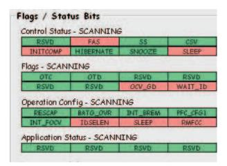
Figure 21. Status Showing Unsealed Mode With Full Access FAS Bit Set
