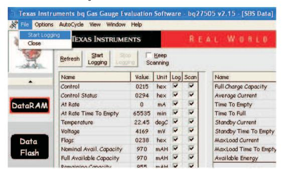
Figure 16. DataRAM Data Logging Command
