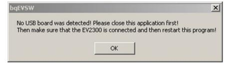
Figure 6. bqEVSW Software Shows No USB Board If EV2300 Is Not Connected
