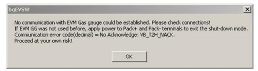
Figure 7. bqEVSW Warns If No EVM or EVM Not Powered Up
