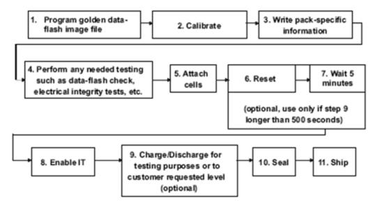
Figure 13. Production Flow Diagram
