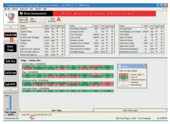
Figure 8. DataRAM Displaying Appropriate Communication With EV2300
