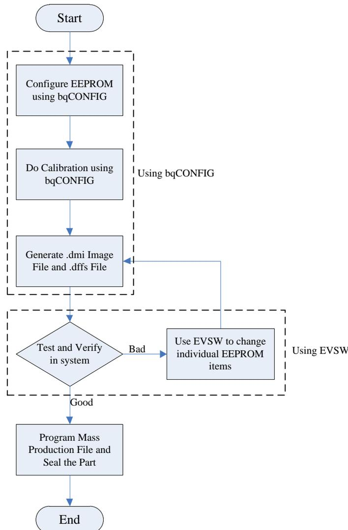
**Figure 1. Flowchart for Creating Mass Production Files**
