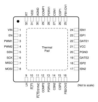
Figure 3. Pin Diagram
