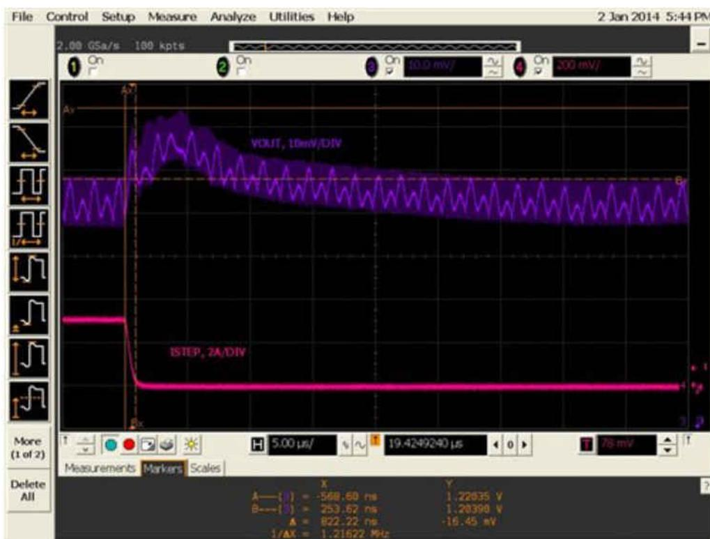
Figure 4-2. Step-Down Load Transient Response
