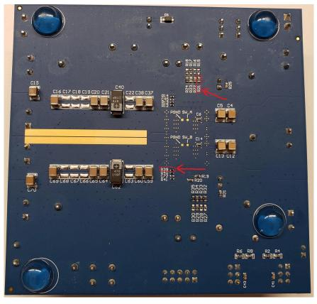
Figure 1-2. Bottom View of TPSM8DC24EVM-2V0 Highlighting R21 and R39
