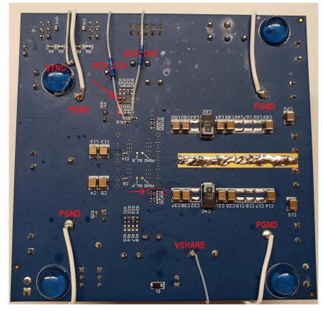
Figure 2-1. Bottom View of Four-Phase Configuration
