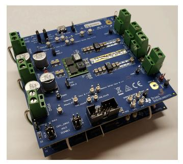
Figure 1-1. 4-Phase Converter Using Two TPSM8D6C24EVM-2V0
