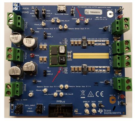
Figure 1-1. Top View of TPSM8DC24EVM-2V0 Highlighting R11 and R26
