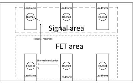
Figure 3-1. Thermal Transfer Direction
