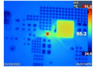
Figure 4-2. TPS566242 12-V Vin to 3.3-V Vout AT 6-A
