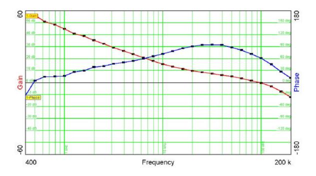
The figure below shows the loop response of the 1.3 V output with a 5.6V input and a 600mA load.
