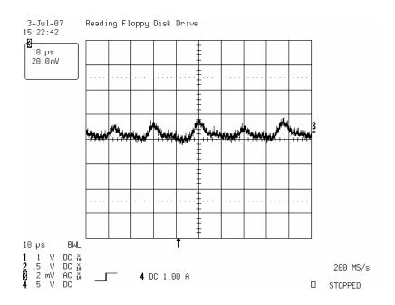
The output ripple voltage of the 1.3V output is shown in the figure below. The image was taken with a 600mA load.
