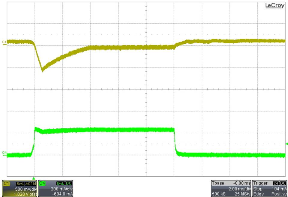
**8.2 30mA to 250mA Transient – 230VAC/50Hz Input**
