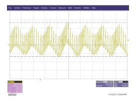
Figure 14 Ripple with 5V,700mA out 265Vac in  $20mV/div\ 500uS/div$
