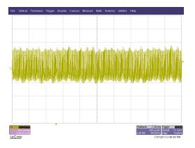
Figure 13 Ripple with 5V,1.2A out 265Vac in  $20mV/div\ 500uS/div$
