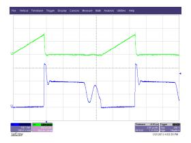
Figure 18 Primary side switching waveforms 85Vac 1.2A load Drain voltage (CH 3 100V/div) IPK voltage (CH4 0.5V/div) 2uS/div
