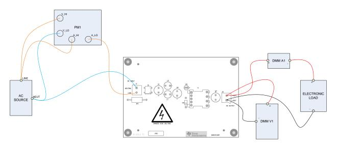
Figure 4. UCC28910FBEVM-526 recommended test set up with a load.
