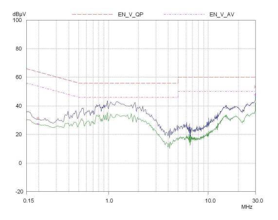
Figure 20. EMI test results per EN55022, Class B.  $115V_{AC}$  input
