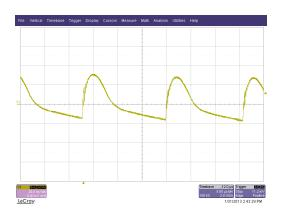
$Figure 12 \ Ripple \ with \ 5V, 1.2A \ out \ 265Vac \ in \ 20mV/div \ 5uS/div$
