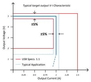
Figure1 Output voltage as a function of output load for the UCC28910EVM-526
