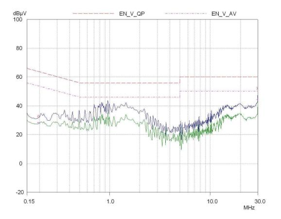
Figure 21. EMI test results per EN55022, Class B.  $230V_{AC}$  input
