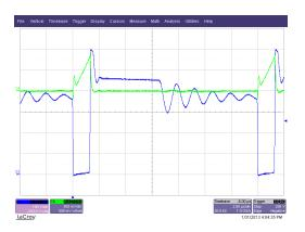
Figure 19 Primary side switching waveforms 265Vac 1.2A load Drain voltage (CH 3 /div) IPK voltage (CH4 /div) 2uS/div
