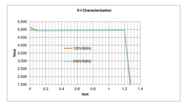
Figure6. Typical V-I Characteristic at 25°C
