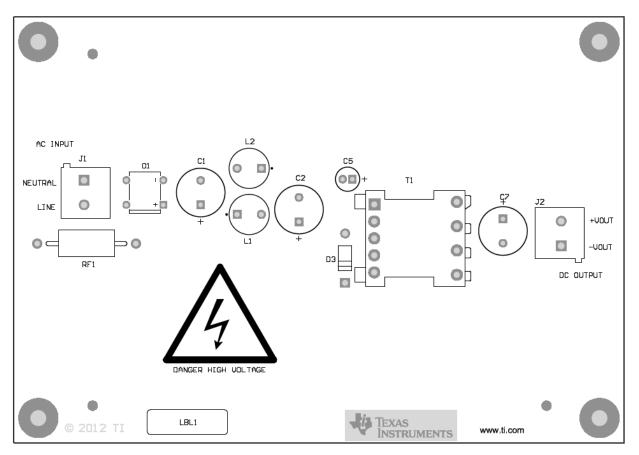
Figure23. Top layer component placement.
