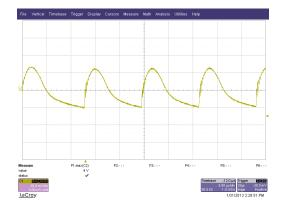
Figure 10 Ripple with 5V,1.2A out 85Vac in 20mV/div 5uS/div
