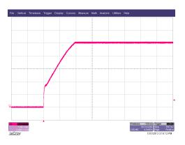
Figure 17 Output voltage start, 230Vac, 1.2A load
