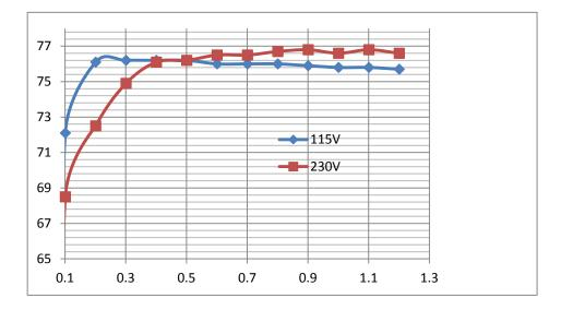
Figure8. Efficiency Vs Iout
