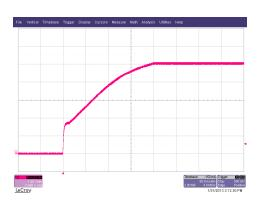
Figure 16 Output voltage start 115Vac,1.2A load
