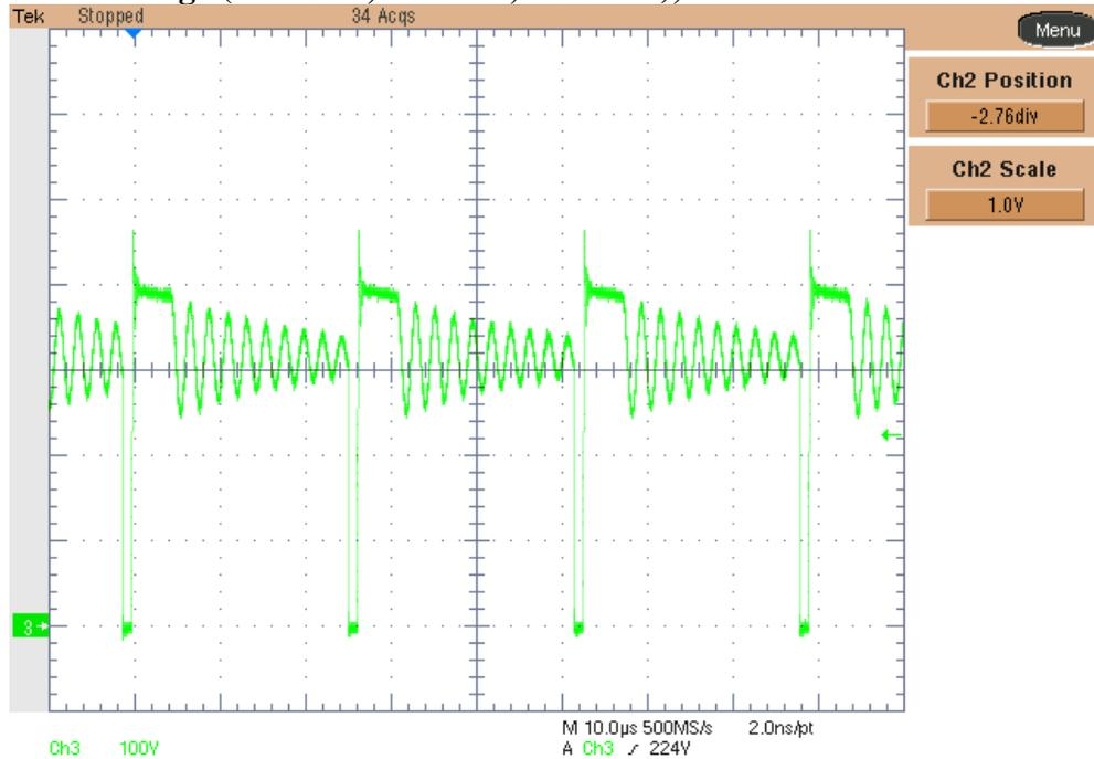
At light load, the converter reduces the switching frequency as shown in the picture below.
