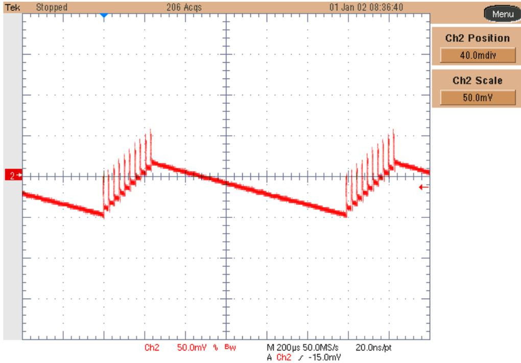
**Ch.2: 17V out (20mV/div, 40us/div, AC coupling, 20MHz BWL), all outputs fully loaded**
