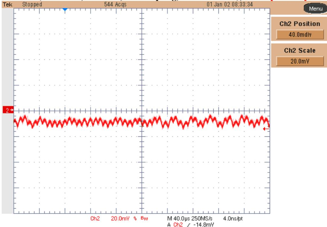
**Ch.2: 23V out (50mV/div, 200us/div, AC coupling, 20MHz BWL), 5% load on all outputs**
