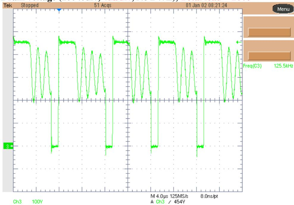
At 5% load on each output the converter enters burst mode:
