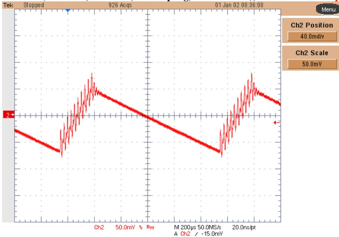
**Ch.2: 23V out (20mV/div, 40us/div, AC coupling, 20MHz BWL), all outputs fully loaded**
