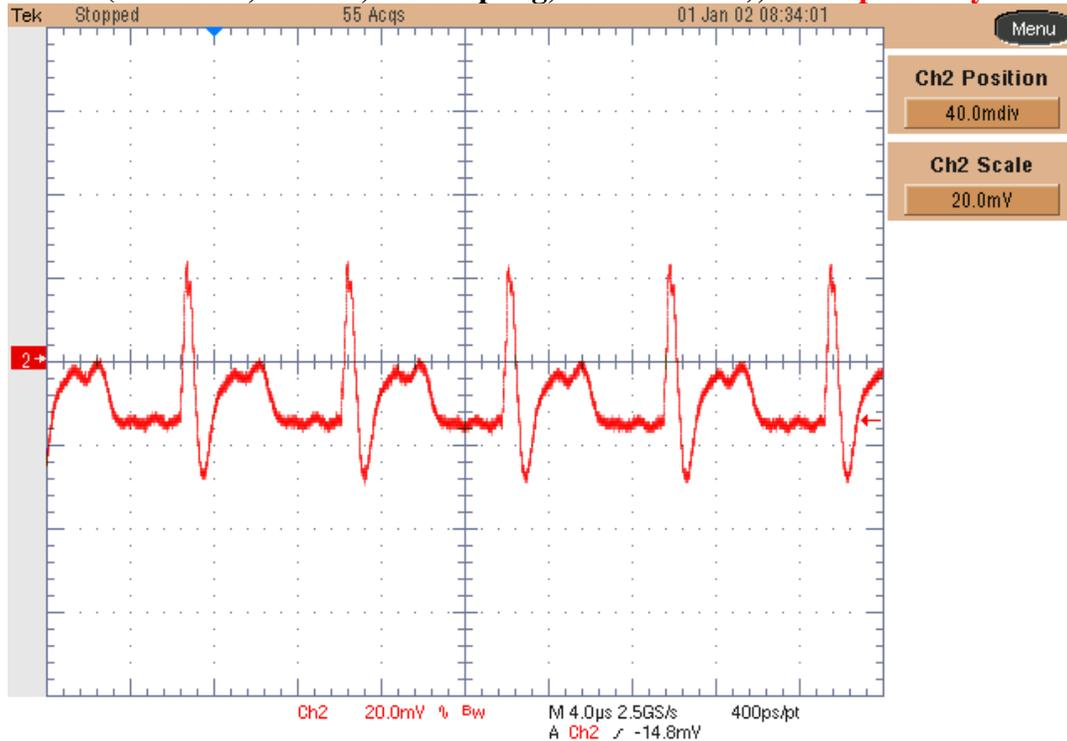
**Ch.2: 9V out (50mV/div, 200us/div, AC coupling, 20MHz BWL), 5% load on all outputs**
