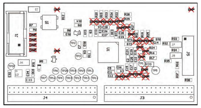
Figure 8. UCD3138ACCEVM149 Top Layer Assembly Drawing (top view)
