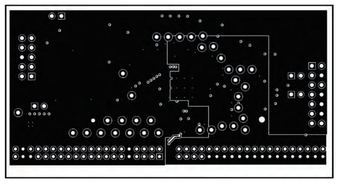
Figure 11. UCD3138ACCEVM149 Internal Layer 1 (top view)
