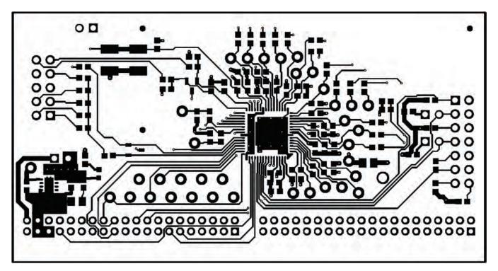
Figure 10. UCD3138ACCEVM149 Top Copper (top view)
