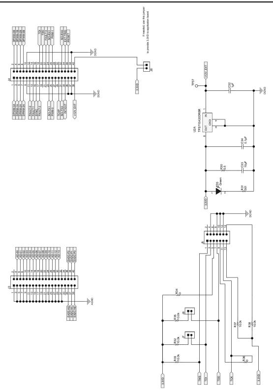
Figure 2. UCD3138ACCEVM149 Schematic (2 of 3)
