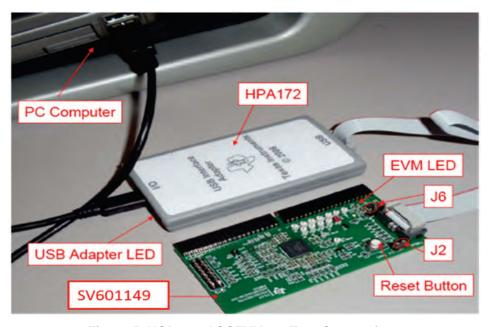
Figure 5. UCD3138ACCEVM149 Test Connections
