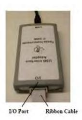
Figure 4. USB-to-GPIO Interface Adapter (HPA172)
