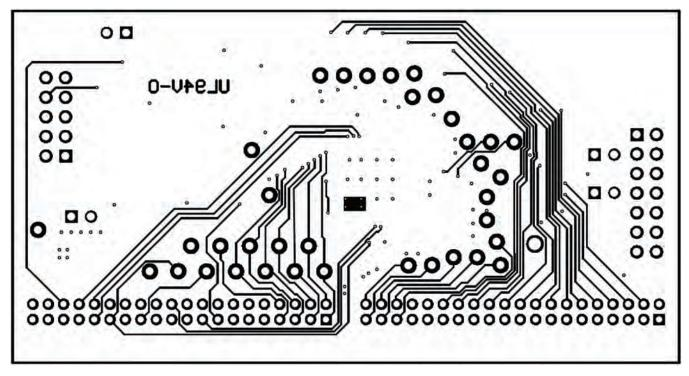
Figure 13. UCD3138ACCEVM149 Bottom Copper (top view)
