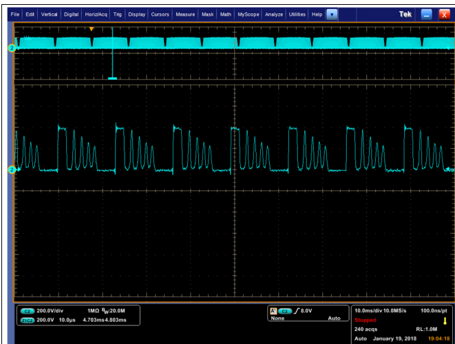
Figure 16. 85 VAC Valley Switching 50-mA Load
