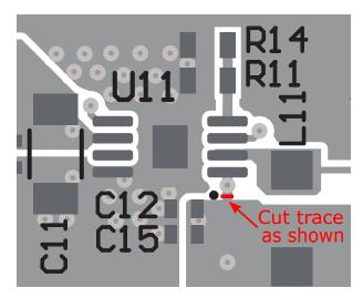
Figure 1. Loop Response Measurement Modification
