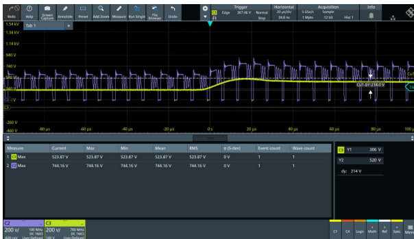
Figure 3-64. 2KV Surge at 230Vac input
