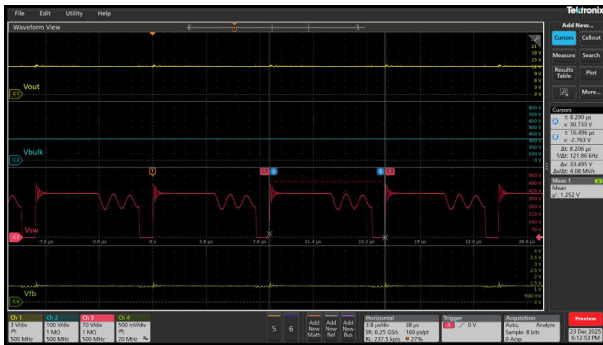
Figure 3-42. 230Vac/27.6W (121kHz frequency / Vfb - 1.252V)
