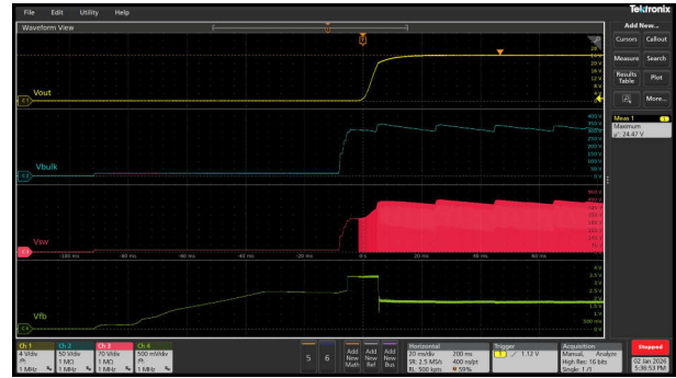
Figure 3-11. Startup waveform for 24V output at full load
