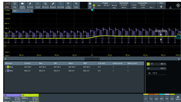
Figure 3-65. 1KV Surge at 230Vac input
