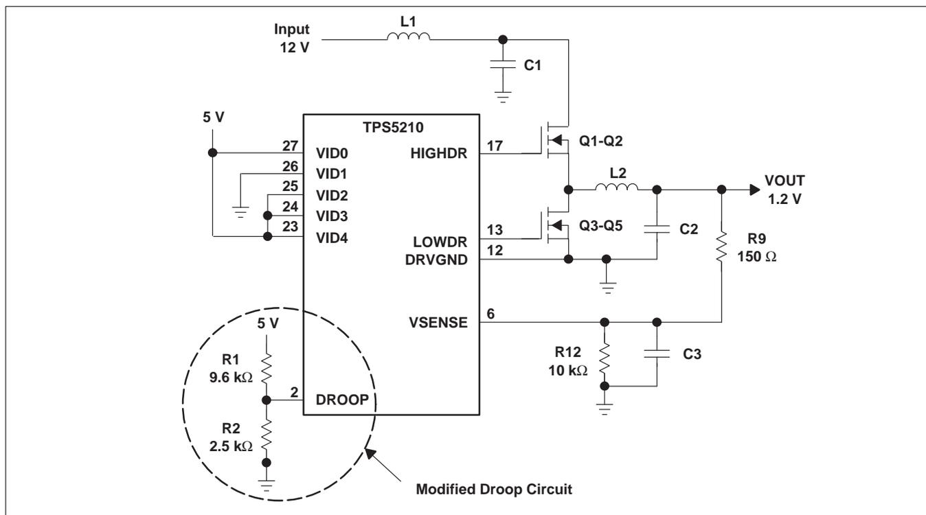
Figure 1. TPS5210 Application Circuit for 1.2-V Output
