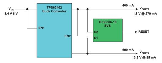
Figure 1. Block Diagram of Power Design
