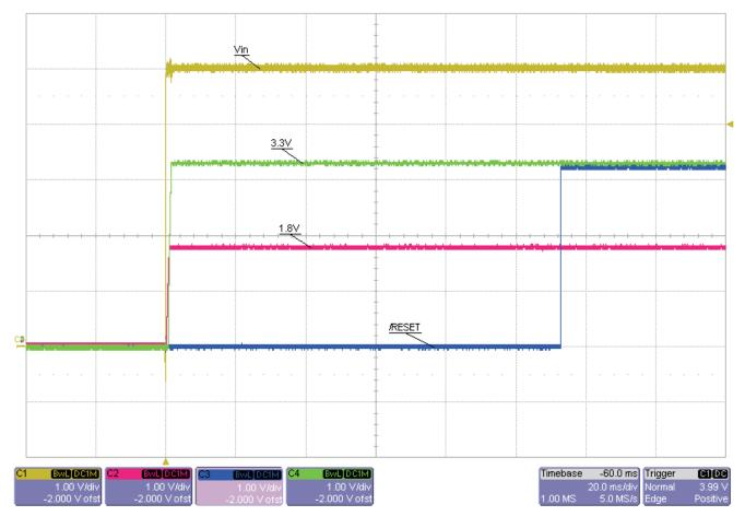
Figure 3. The RESET Signal Held Low for a 100-ms Typical Fixed Delay
