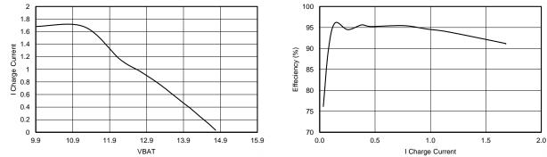
Figure 9. Bench Result of Charge Current vs. Battery Voltage using EVM Modification of TPS5402
