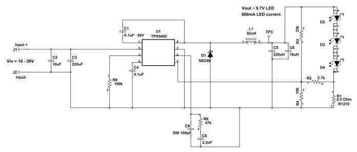
Figure 11. Simple LED Driver Implementation using TPS5402
