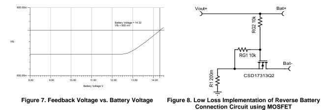
The user is able to also remove the D2 and use a MOSFET in the configuration shown in Figure 8 to improve efficiency. A lower  $R_{dson}$  MOSFET ensures better efficiencies at higher charge currents.
