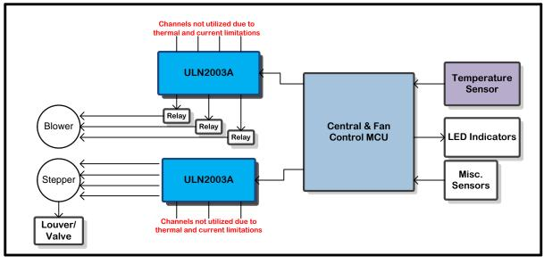
Figure 7. Air Conditioning System Using Two ULN2003A Chips to Drive Peripherals
