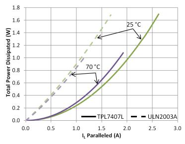
Figure 5. Dissipated Power Versus Seven Paralleled Channel Output Current for TPL7407L and ULN2003A
