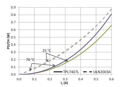
Figure 4. Dissipated Power per Channel Versus Output Current for TPL7407L and ULN2003A
