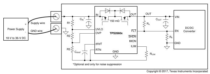
Figure 1. TPS2660 Power Good Indication Using FLTb
