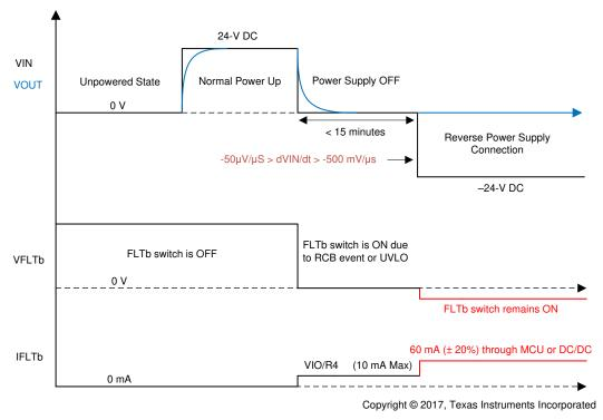
Figure 4. Power Supply Sequence Where FLTb Sinks More Current
