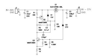
Figure 2-2. Discrete Voltage Clamping Circuit
