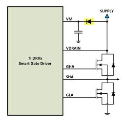
Figure 1. Modified Circuit with Diode
