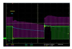
Figure 3. Momentary Turn Off With Diode
