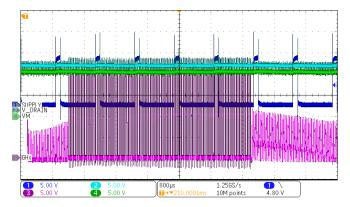
Figure 4. Recurring Voltage Drops with Diode
