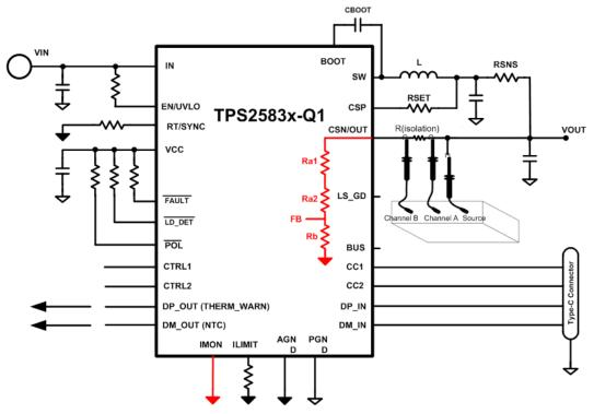
Figure 3. Setup of Loop Test
