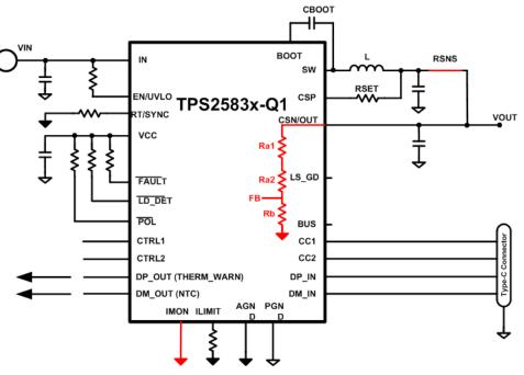
Figure 1. TPS2583x-Q1 System Without Cable Compensation Function
