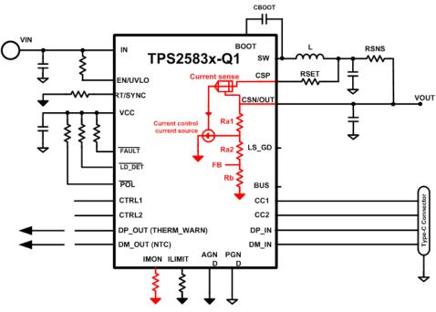
Figure 2. TPS2583x-Q1 System With Cable Compensation Function
