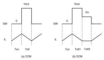
Figure 2-1. Waveforms of Boost SW Voltage in CCM and DCM
