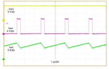
Figure 3-5. TPS61089 Power Vin = 1.5 V, Signal Vin = 3.6 V, Vo = 9 V, Io = 1 A
