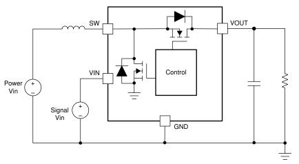
Figure 1-2. External Bias Application of Synchronous Boost Converter
