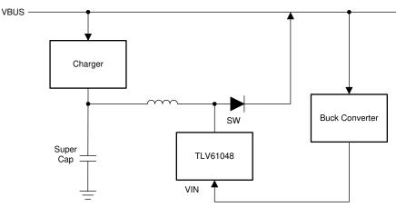
Figure 4-1. Simplified Block Diagram of Backup Power Supply
