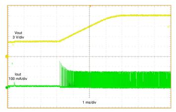
Figure 2-2. TLV61046a Power Vin = Signal Vin = 5 V, Vo = 12 V, Io = 10 mA, Power Vin Provided First
