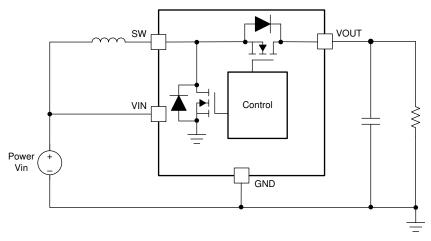
Figure 1-1. Typical Application of Synchronous Boost Converter
