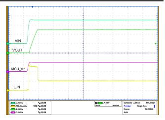
Figure 7. Successful Startup with a Reset Signal from MCU
