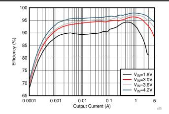
Figure 1. TPS61022 Load Efficiency with Different Input in Auto PFM
