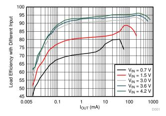
Figure 2. TPS61099 Load Efficiency with Different Inputs
