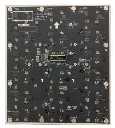
Figure 2-4. The Back of the LED Panel Module Prototype Board (96 × 108)
