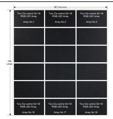
Figure 2-3. The Front of the LED Panel Module Prototype Board (96 × 108)
