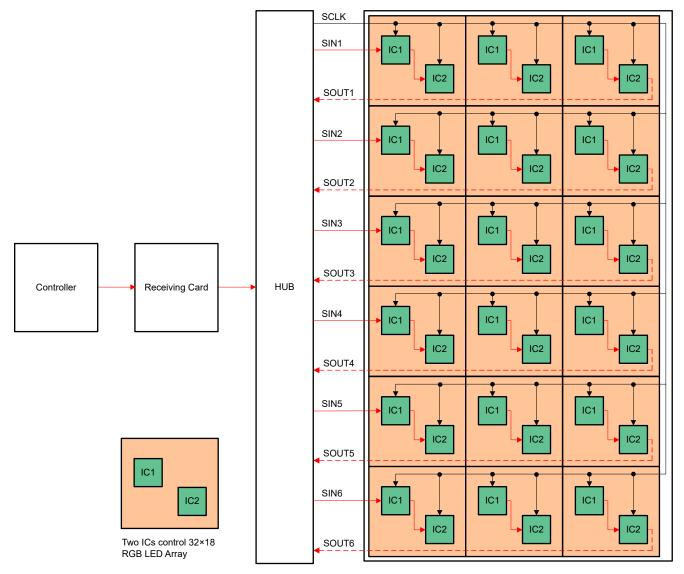
Figure 2-2. Details of the LED Panel Module (96 × 108)
