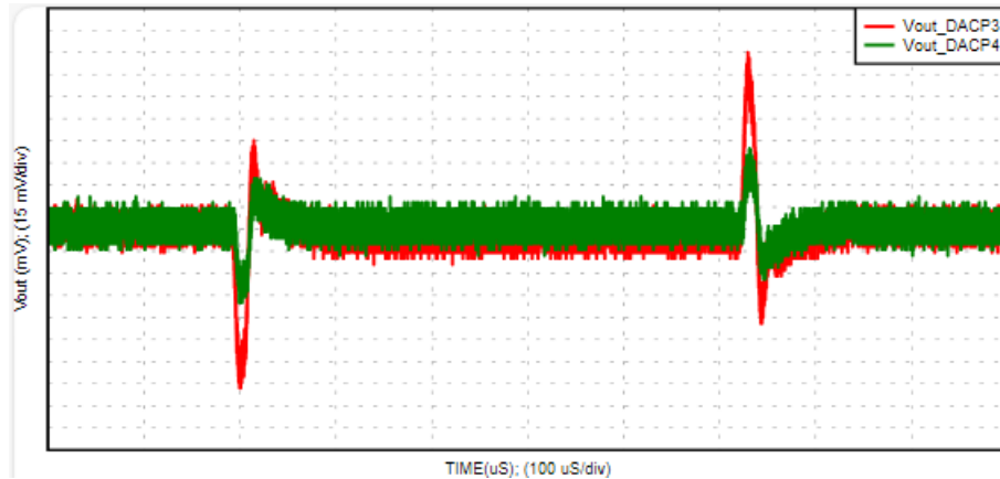
Figure 5. D-CAP4™ versus D-CAP3™ Transient Performance
