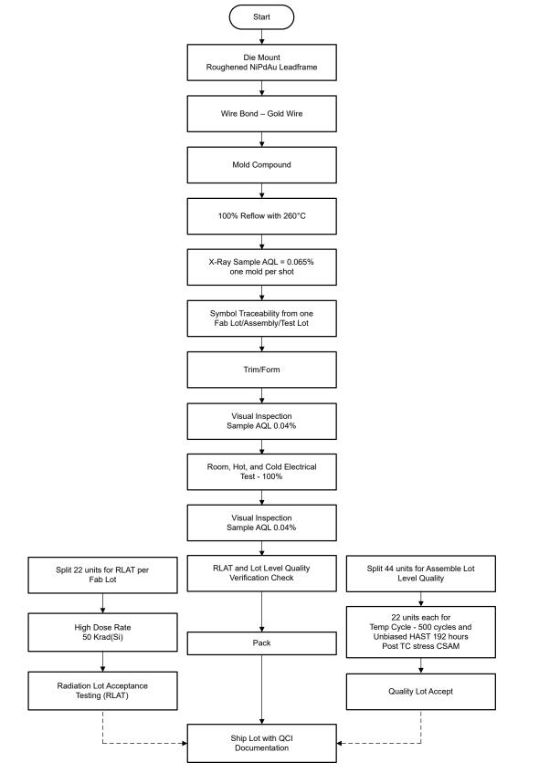
Figure 2-1. TPS7H500x-SEP Space Enhanced Plastic Production Flow Chart
