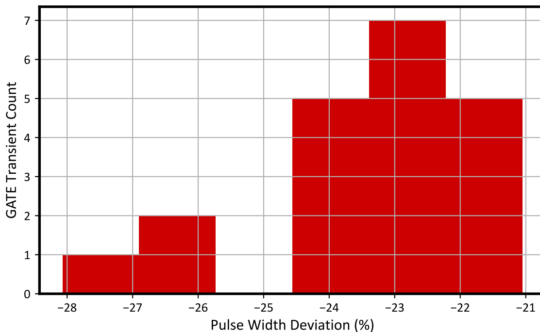
Figure 8-2. TPS7H5020-SEP Silicon Mode GATE Pulse-Width Deviation Histogram (Run #19)
