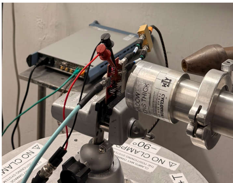
Figure 4-1. Decapped TRF0108-SEP Evaluation Board Mounted in Front of the Heavy-Ion Beam Exit Port
