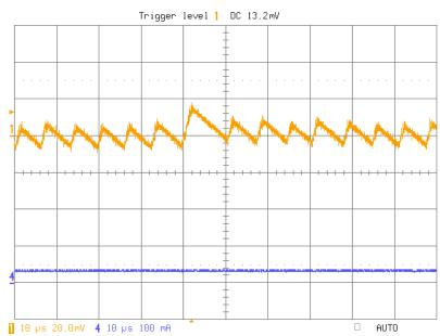
Fig 6: Output ripple on 3.3V @ 0.04A with 6Vin (high line), Ch1: Output ripple, Ch4: Output load
