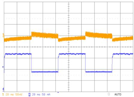
Fig 10: 50% to 100% transient 3.3V @ 0.165A output with 3.6Vin. Ch 1: 3.3V output; Ch 4: Load current
