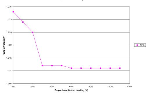
Fig 16: Load regulation on 1.2V output, 3.3V output is proportionally loaded
