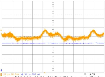
Fig 5: Output ripple on 1.2V @ 0.66A with 6Vin (high line), Ch1: Output ripple, Ch4: Output load
