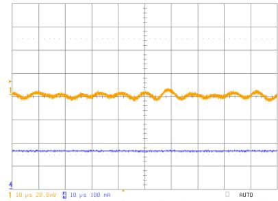
Fig 4: Output ripple on 3.3V@ 0.165A with 3.6Vin (Low Line), Ch1: Output ripple, Ch4: Output load
