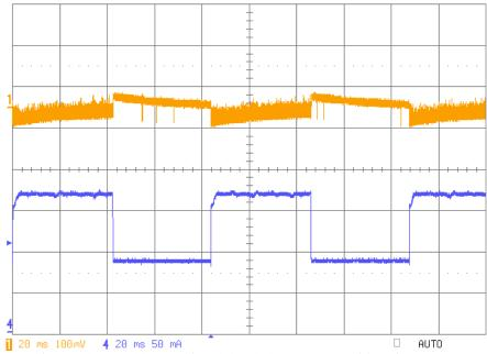
Fig 12: 50% to 100% transient 3.3V @ 0.66A output with 6Vin. Ch 1: 3.3V output; Ch 4: Load current
