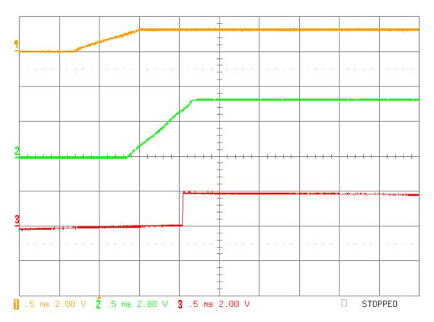
Fig 2: Start up waveform with all outputs fully loaded
