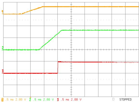
Fig 1: Start up waveform with outputs unloaded
