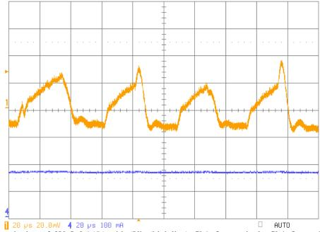
Fig 7: Output ripple on 3.3V @ 0.165A with 6Vin (high line), Ch1: Output ripple, Ch4: Output load
