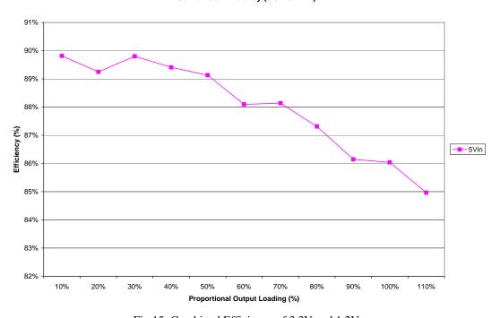
Fig 15: Combined Efficiency of 3.3V and 1.2V
