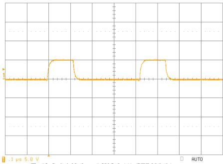
Fig 13: Switch Node on 1.2V@ 0.66A (PWM Mode)
