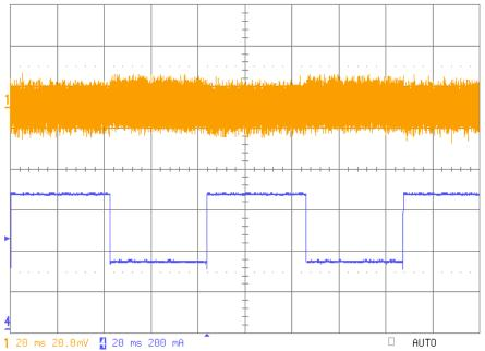
Fig 11: 50% to 100% transient 1.2V @ 0.66A output with 6Vin. Ch 1: 1.2V output; Ch 4: Load current
