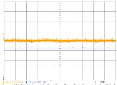
Fig 3: Output ripple on 1.2V @ 0.66A with 3.6Vin (Low line), Ch1: Output ripple, Ch4: Output load
