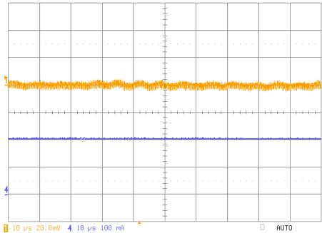
Fig 8: Output ripple on 3.3V @ 0.2A with 6Vin (high line), Ch1: Output ripple, Ch4: Output load
