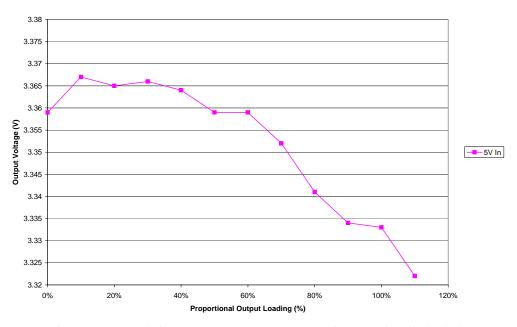
Fig 17: Load regulation on 3.3V output, 1.2V output is proportionally loaded
