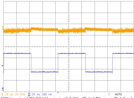
Fig 9: 50% to 100% transient 1.2V @0.66A output with 3.6Vin. Ch 1: 1.2V output; Ch 4: Load current
