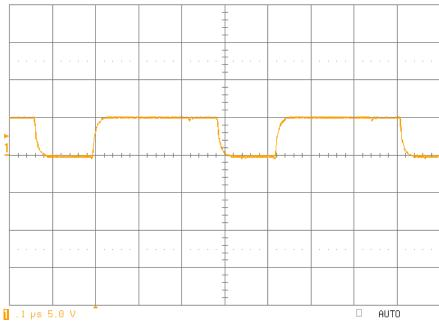
Fig 14: Switch Node on 3.3V@ 0.2A (PWM Mode)
