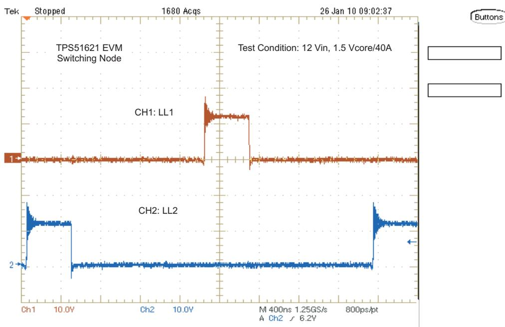
Figure 11. TPS51621EVM-602 Switching Node at 40 A
