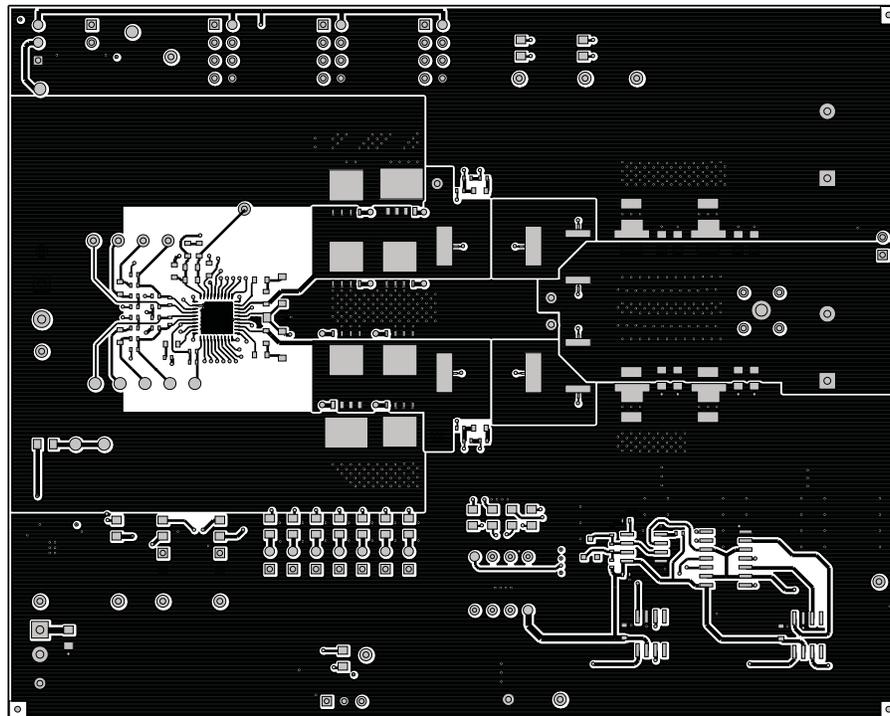
Figure 22. TPS51621EVM-602 Top Copper, Top View
