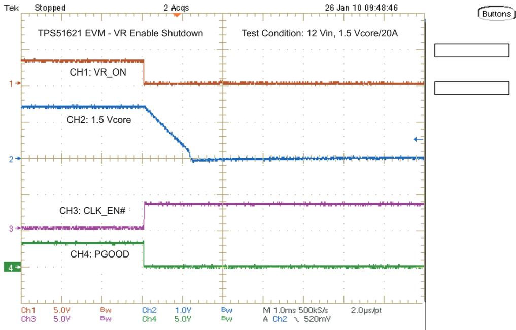
Figure 17. TPS51621EVM-602 Enable Turns Off Waveform
