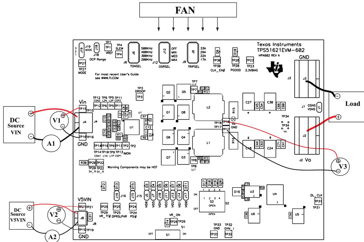
**Figure 4. TPS51621EVM-602 Recommended Test Setup**
