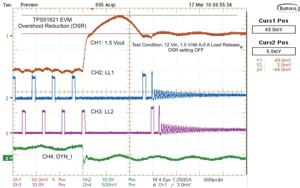
Figure 14. TPS51621EVM-602 Output Transient Release Without Overshoot Reduction
