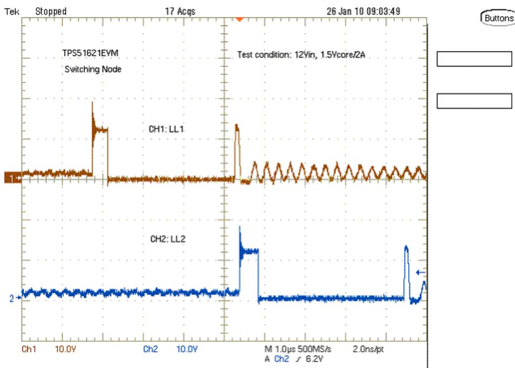
Figure 12. TPS51621EVM-602 Switching Node at 2 A
