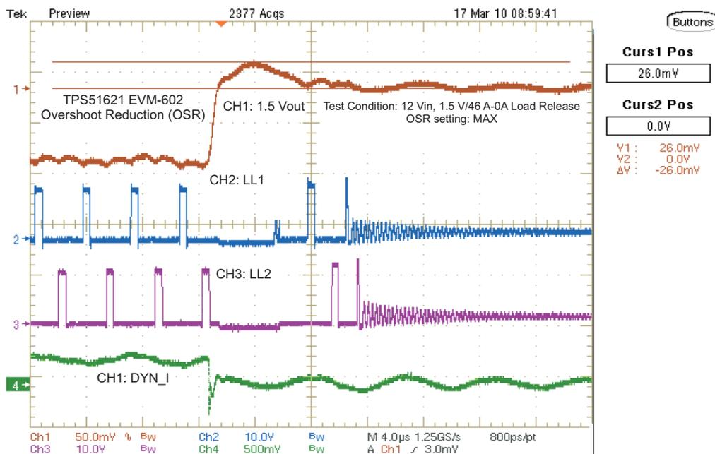
Figure 15. TPS51621EVM-602 Output Transient Release With Maximum Overshoot Reduction
