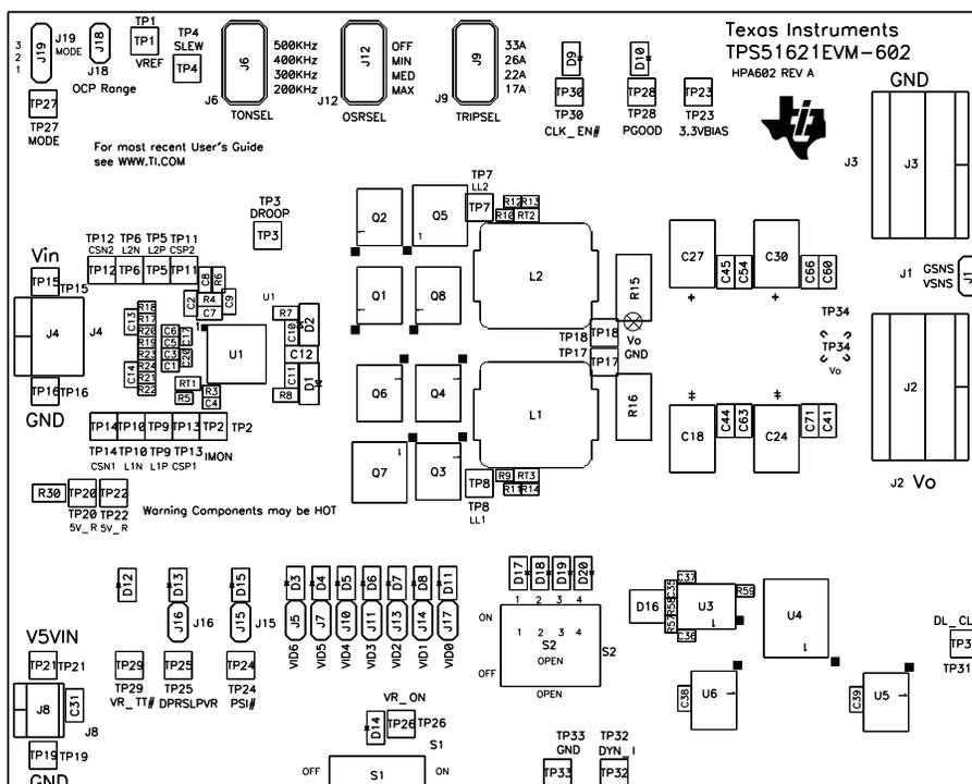
Figure 20. TPS51621EVM-602 Top Layer Assembly Drawing, Top View
