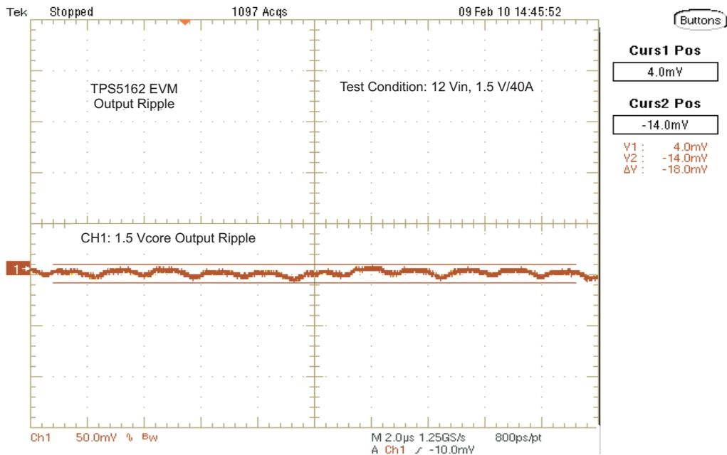
Figure 10. TPS51621EVM-602 Output Ripple
