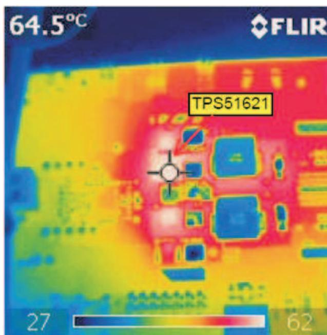
Figure 19. TPS51621EVM-602 Top Side Thermal Image, Test Condition: 12 Vin, 1.5 V/40 A
