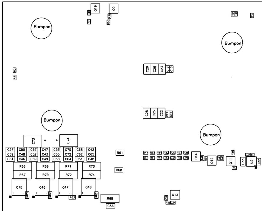
Figure 21. TPS51621EVM-602 Bottom Assembly Drawing, Bottom View
