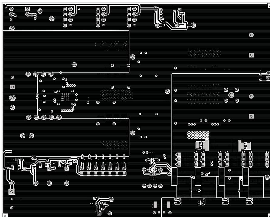
Figure 27. TPS51621EVM-602 Bottom Layer, Top View
