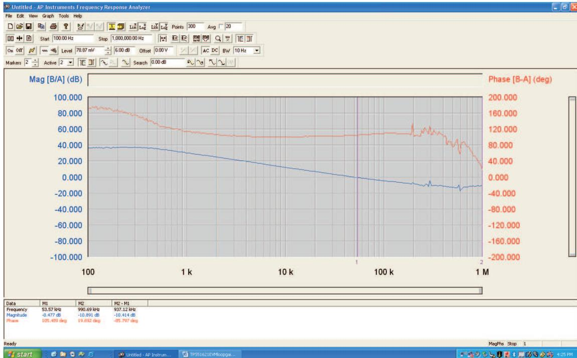
Figure 18. TPS51621EVM-602 Bode Plot, Test Condition: 12 Vin, 1.5 V/40 A
